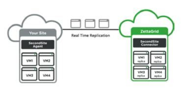
SecondSite<sup>™</sup> utilises Virtual Protection Group (VPG) technology to recover financial applications that consist of multiple VMs together to the same point in time, ensuring a consistent recovery. Without a VPG, the recovery of applications can be broken, as each VM could be recovered to different points in time and potentially referencing financial data that is not present in all of the applications and VMs recovered.
